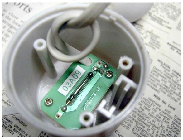
Thinking there was probably a magnet on a shaft coming into this chamber from the cups on top, I removed the PCB:
