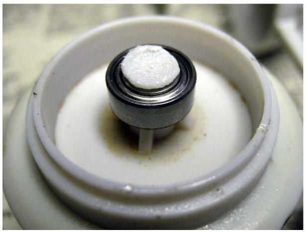
I sprayed the bearing with WD-40 and spun it round many times to ensure it was running freely.
