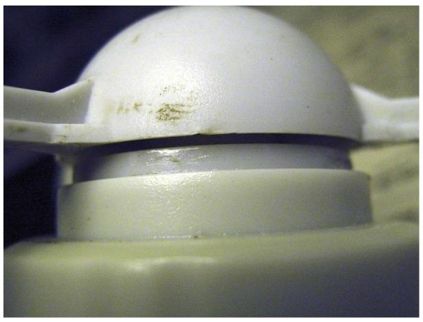
At this stage I used a bit of brute force and stuck a small screwdriver under the 'cap' and levered it up while pushing up on the other side with a finger (you can see some of the resulting 'dints' in the photos!). A bit more of this and the cap popped off, revealing...
