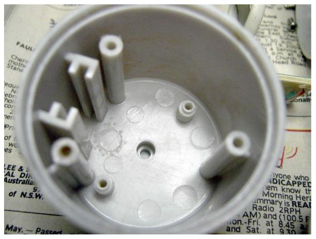
But there was no connection between the cups and the 'electronics' chamber (that 'hole' at the top [this photo has the chamber upside-down] is sealed).
