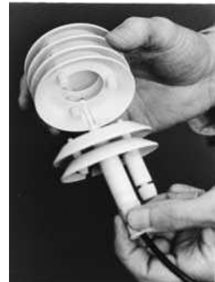
Two-part construction allows easy access for cleaning.
