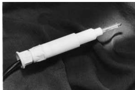
Hard glass prt element with holder containing thermal barrier and lead resistance equalization.
